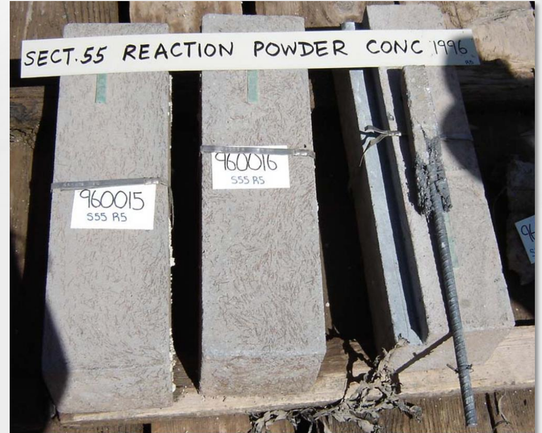
In 2006 – Rebar at 10-mm (3/8-inch) cover removed from one of the 10-year-old beams
